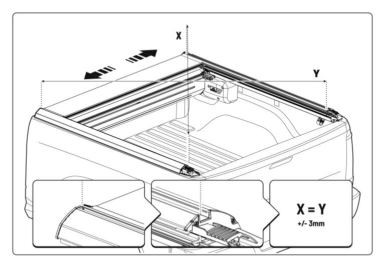
• Ensure the cross measurements are identical.
