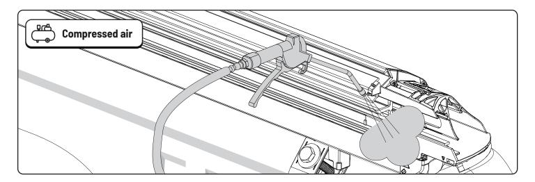
Remove dirt and debris using compressed air.
